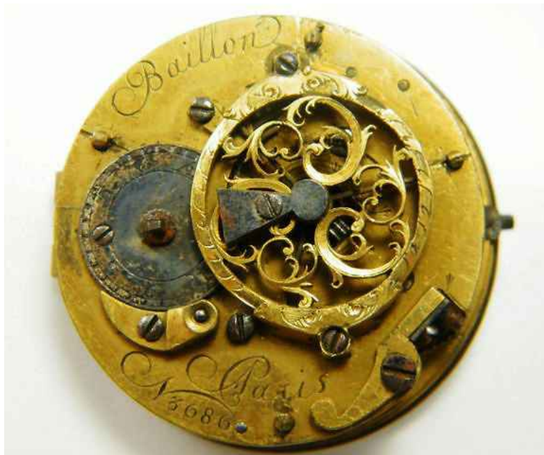
Figure 3 Baillon Watch movement with probable verge escapement
